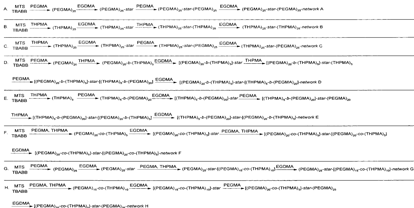
Figure 2. Synthetic sequences employed for the preparation of the various cross-linked star architectures of this study: PEGMA, methoxy poly(ethylene glycol) methacrylate; THPMA, tetrahydropyranyl methacrylate; EGDMA, ethylene glycol dimethacrylate; MTS, 1-methoxy-1-(trimethylsiloxy)-2-methylpropene; TBABB, tetrabutylammonium bibenzoate.
